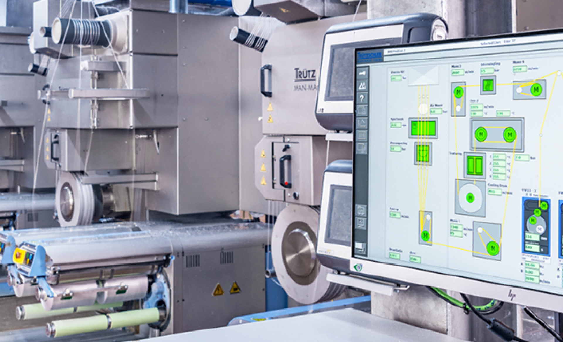
Figure: Trützschler Central Monitoring Unit (CMU) system combines all functionalities to control the extrusion line. Courtesy: ategroup.com
