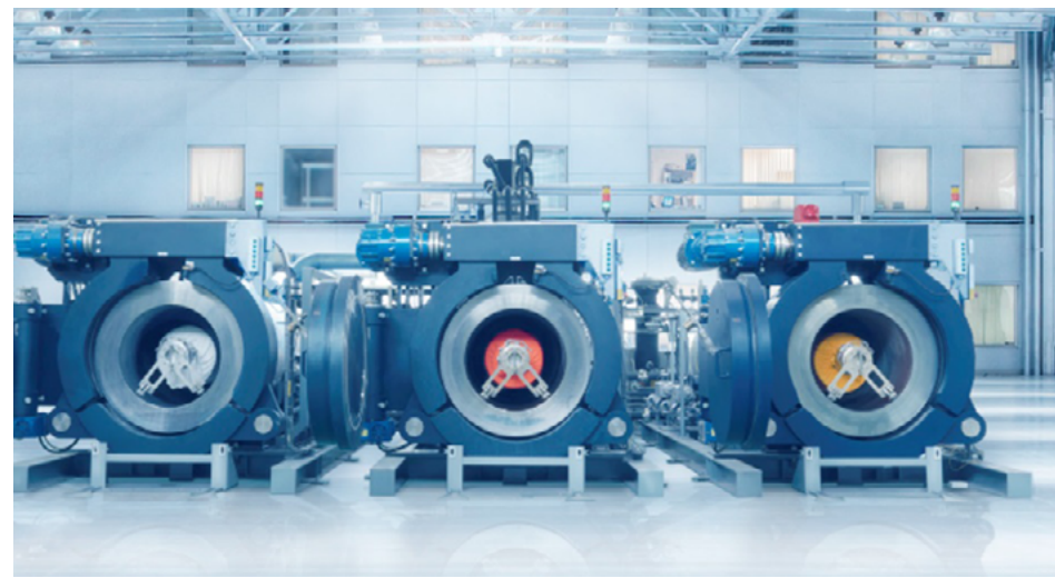
Figure 4: DyeCoo Textile Systems has developed a breakthrough technology for yarn and fabric dyeing using carbon dioxide (CO 2 ) as the dyeing medium.
