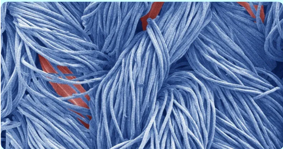
Figure: Textile fibers (blue) can be given a uniform water-repellent finish using plasma coating. Even more demanding elastic fibers (red) remain permanently impregnated thanks to the new process. (Scanning electron microscopy, colored) Image: Empa
