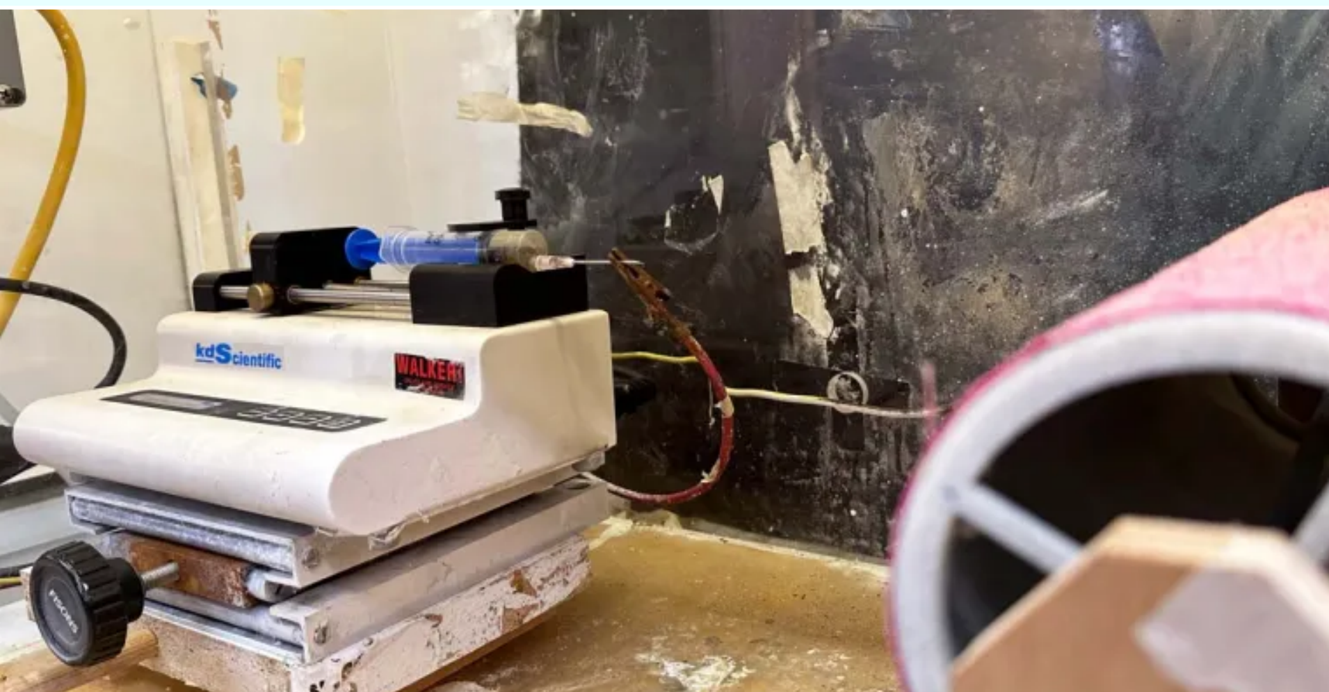
The electrospinning machine created a web of nanofibres on the cotton fibres, which are then cured to bond the two. Credit: Cherry Cai, RMIT University
