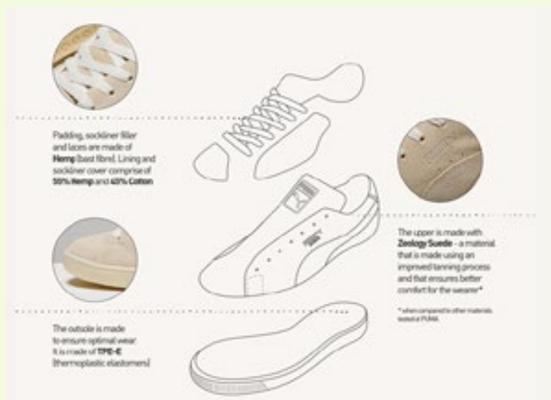
Fig. Diagram of the materials within RE:SUEDE sneakers. Source: Puma
